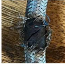
Broken fibres visible
